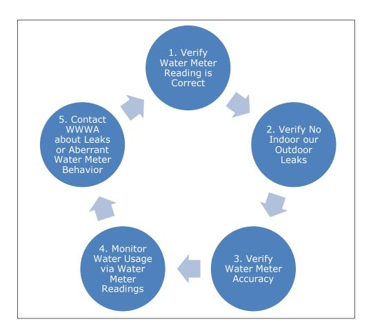
1. <u>Verify Water Meter Reading is Correct.</u> Visually inspect the water meter and write down the meter reading. Compare that observed number to the number recorded on the received water bill.
